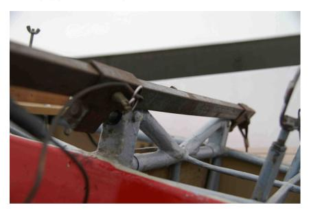
...and the shackle of the outboard cable is secured to the eye on the outside trailer tube. The stabiliser bar cables are then tightened to support the fuselage by tightening the turnbuckles on either side. *Do not overtighten*.
