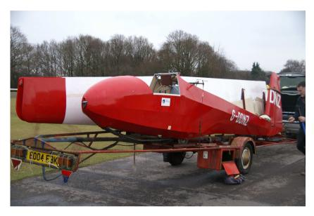
This needs one person on the tail and 3 to lift the nose; it helps to have one person standing on the trailer to help take the weight of the cockpit. Lift by holding only fixed tubes or the nose skid. The wheel goes in a cradle and the tailskid in its holder.
