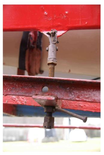
28. Tie up aileron and airbrake connections to stop them thrashing around (using bungee provided):
