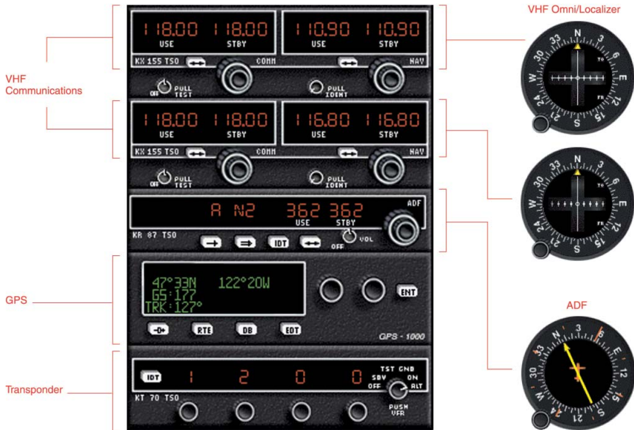
Figure 9-1. Typical NAV/COM Installation.
