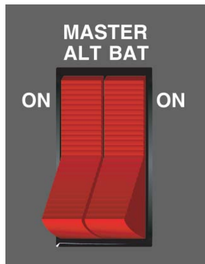
Figure 11-5. Double Rocker Switch Seen on Many Aircraft.
