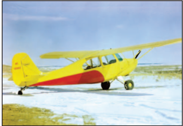
Figure 5-27. Tailwheel landing gear.
