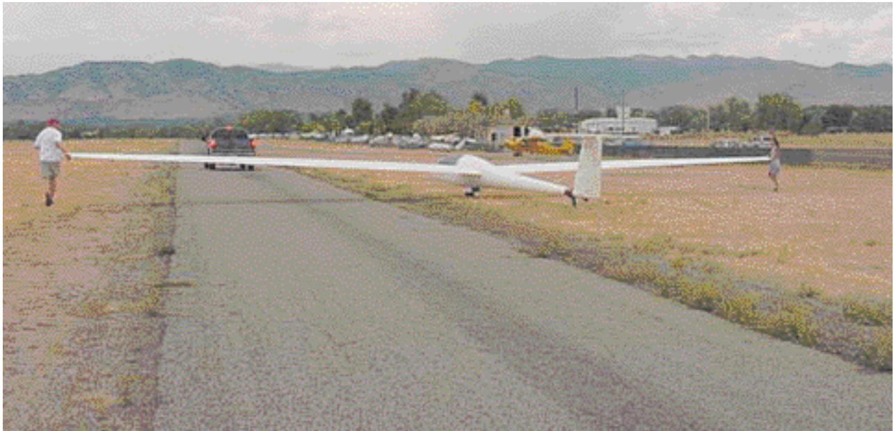
Figure 6-5. Positioning the glider for the tow vehicle.
