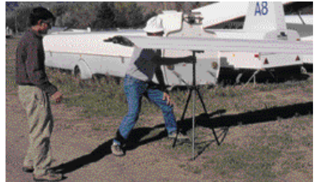
Figure 6-1. Wing stand used during glider assembly.
