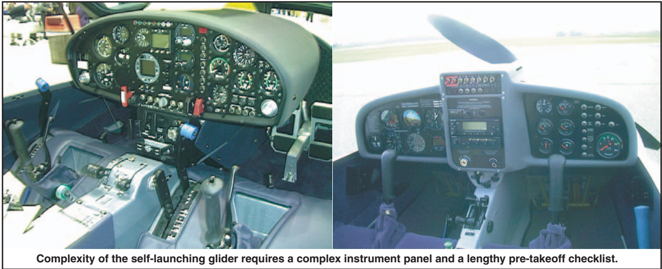
Figure 7-22. Self-launch glider instrument panels.
