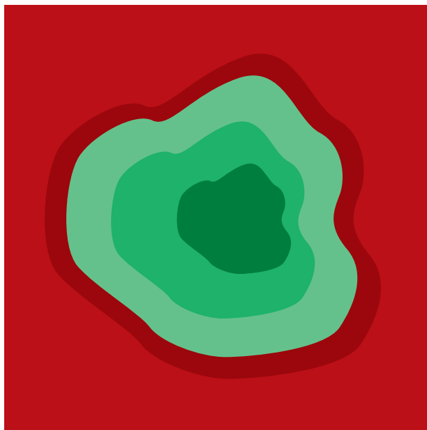
Figure 9-7. Cross-section through a thermal. Darker green is stronger lift, red is sink.
