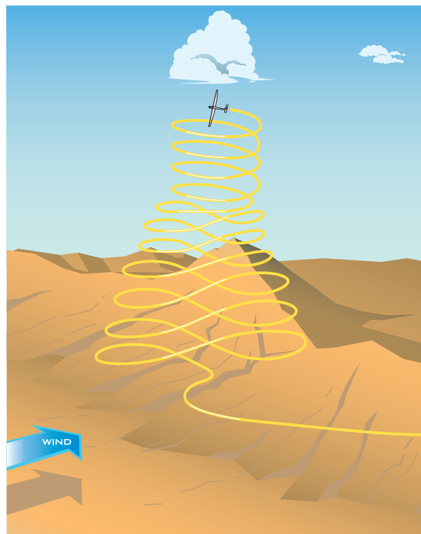
Figure 10-17. One technique for catching a thermal from ridge lift.
