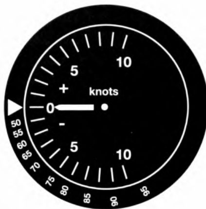
Fig A1.2 Marking up a speed-to-fly ring.
