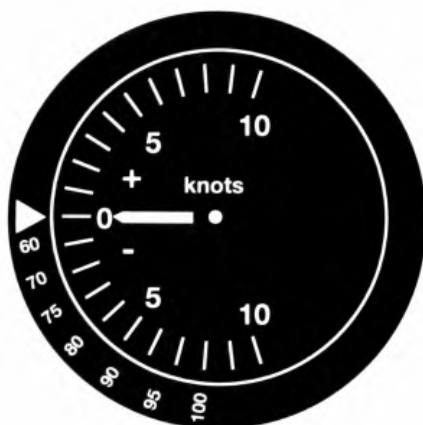
Fig A1.3 Speed-to-fly ring – calibrated for air mass.
