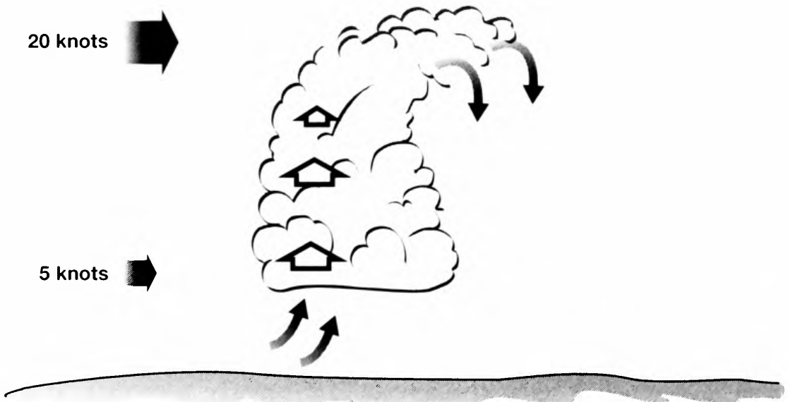
Fig 3.4 Toppling cumulus. Stronger winds aloft may cause clouds to topple downwind as they decay. Any lift will be towards the upwind side.
