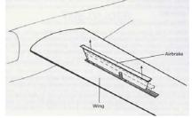
drag to stop the glider exceeding its maximum speed in a vertical dive. Higher performance modern gliders are too efficient by comparison to the older designs so now manufacturers only achieve this speed limiting capability in up to 45° dives. Still, this is a very useful safety feature.
