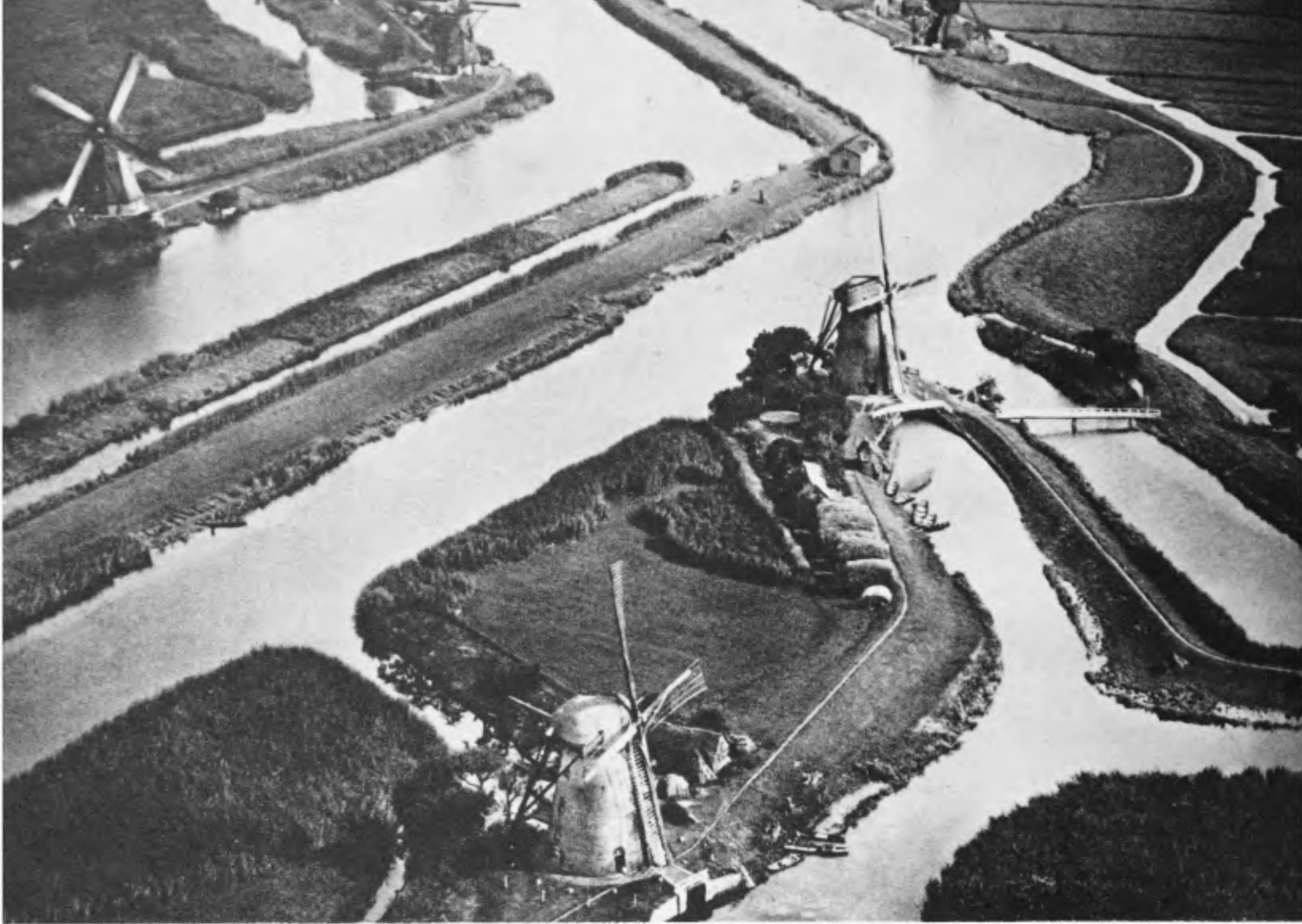
4 For centuries the "windmills" of Holland have worked night and day. Wind, water, earth, sea, such are the given factors of the problem. And for centuries, with- out ceasing, the water of the 'polders' (land below sea-level) has been pumped into the canals (above sea-level).
