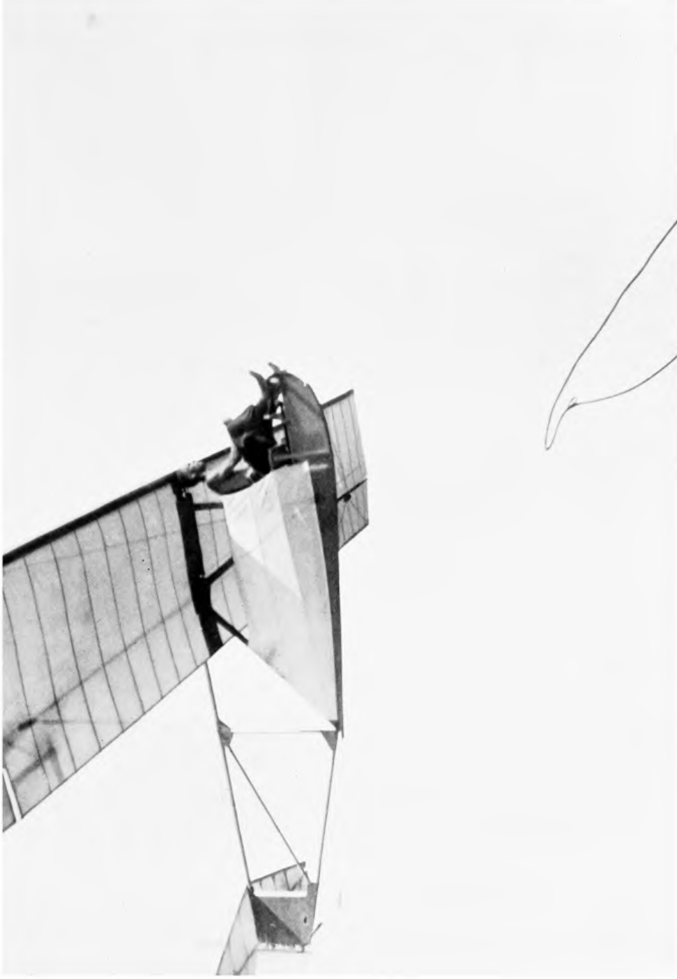
71. A "ZÖGLING" IN THE AIR. NOTE THE OPEN SEAT AND THE SIMPLICITY OF THE MACHINE'S CONSTRUCTION
