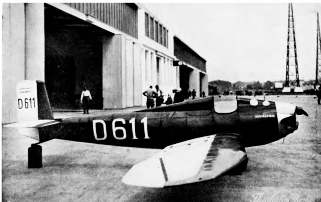
24. THE DARMSTADT ACADEMIC FLYING GROUP'S "MOHAMED," A TYPICAL DESCENDANT OF THE SOARING PLANE FITTED WITH A LIGHT ENGINE
