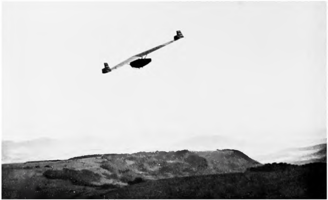
4. THE RHÖN-ROSSITTEN COMPANY'S TAILLESS SOARER, THE "STORCH," WHICH WAS GIVEN A LIGHT ENGINE FOR A SERIES OF EXPERIMENTS
