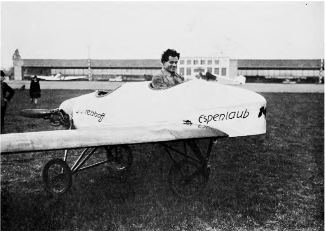
20. SOLDENHOFF'S TAILLESS MOTOR-PLANE. BUILT AND FLOWN BY ESPENLAUB, THE WELL-KNOWN SOARING FLYER
